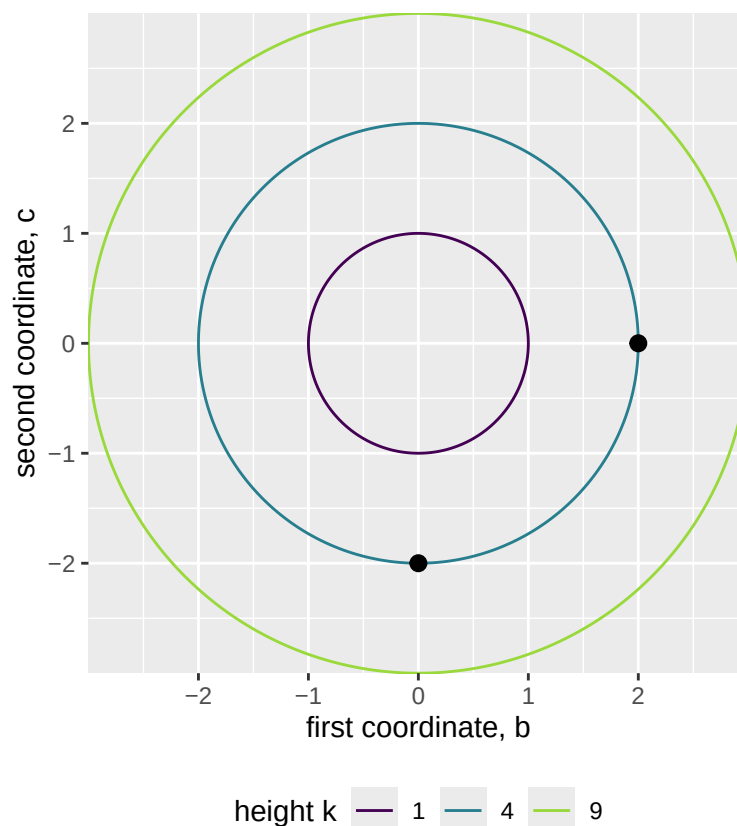
Figure 1: The contour lines of g(b, c) = b^2 + c^2 at heights 1, 4 and 9. The dots mark the points (2, 0) and (0, -2) of the example on the circle at height 4.
